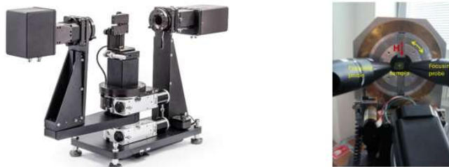
Spectroscopic ellipsometer WOLLAM RC2-DI used for thin film characterization (left), rotating permanent magnet circuit for magneto-optical characterization (right).
